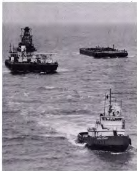
ALL-OCEAN TUG, MISTER RICHARD, equipped with two ALCO, V-12, 251s rated at 2650 BHP each has 13 knots free-running speed.
