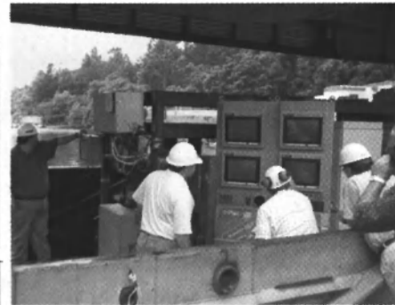
"Bridge Control Interface" - Built to operate reliably in "rollover" conditions, Bridge Control Interfaces are fully sealed and feature "hibrite" displays for daylight viewing.
