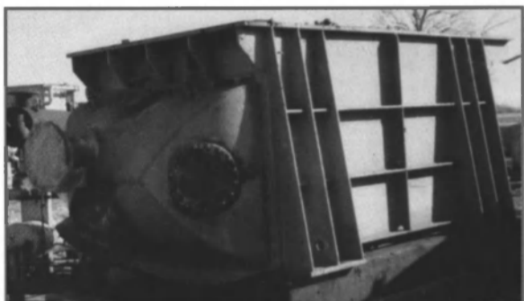
1 Unused Main Condenser Mfg: C.H. Wheeler 3800 sq. ft. | Pass 2446 Tubes of 5/8" OD and 0.049" Wall Thickness CuNi 70-30 9'8 1/8" Long Waterboxes of CuNi & Tube Sheets 180"x96"x92"High 18"Swing Bronze Check Valve on Ea. Unit
