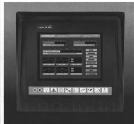
"Bridge Control Interface" - Built to operate reliably in "rollover" conditions, Bridge Control Interfaces are fully sealed and feature "hibrite" displays for daylight viewing.
