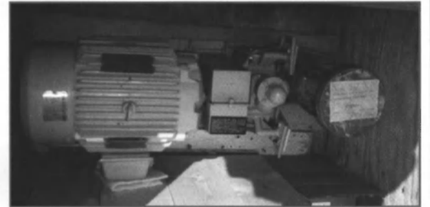
15 Foam Fire-Fighting Pumps Mfg: Blackmer 35GPM@200psi Horizontal Model BXL1/25NFC-TB Motor: Reliance 7.5HP 440/3/60 With Controller, Spares and Educator Assembly
